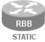
RBB is a backbone router with a static configuration. At least one Fast Ethernet port supporting 802.1q is required. NETLAB<sub>AE</sub> does not allocate an access server connection for RBB, so users cannot directly access the console port. However, it is part of the topology so users can indirectly interact with it (i.e. ping, trace, RIP, etc.).
